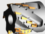
05 Walter milling tool for angled cheek faces
