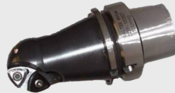
03 Walter Modco Motion tool for cylinder bore finish
