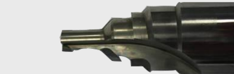
02 Walter PCD boring bar to rough parent metal bore
