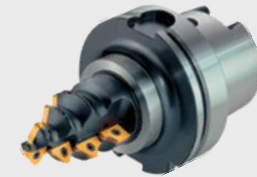
08 Walter indexable form cutter for finishing of fir tree slots
